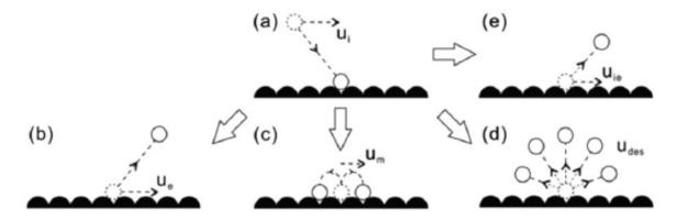
Fig. 1 Molecular interaction at a fluid-solid interface: (a) incident molecule, (b) elastic scattering, (c) surface hopping, (d) desorption and (e) inelastic scattering.
