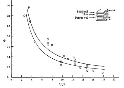
FIGURE 4.  $\Phi$  as a function of  $h/\sqrt{k}$  for foametal porous specimens using demineralized water.  $k = 1.1 \times 10^{-5}$  in.<sup>2</sup>. Curve P,  $\alpha = 0.8$ ; curve Q,  $\alpha = 1.2$ .
