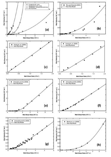
Fig. 3 Validation of the new slip model (solid lines) for liquid-solid interfaces using experimental results (symbols) from the literature. The fitting coefficients are summarised in Table 2.
