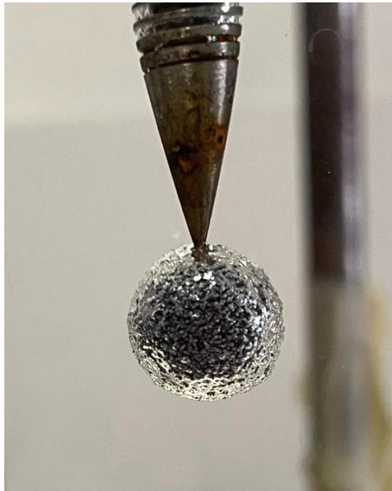
*Figure 1-11 Sphere with superhydrophobic coating in a water tank hold by an electromagnetic holder.*
