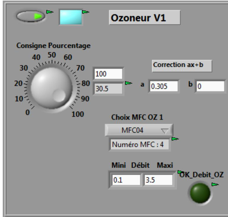
Figure 4.1: *Labview interface to control ozone production.*
