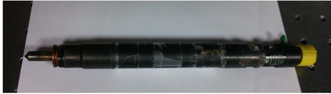
Figure 2.3: *Delphi Diesel Injector.*
