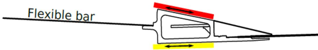
Figure 3.4: Trailing edge sliding mechanism
