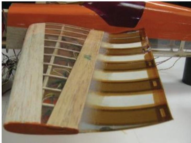
Figure 1.7: MFC applied to the trailing edge of wing model
