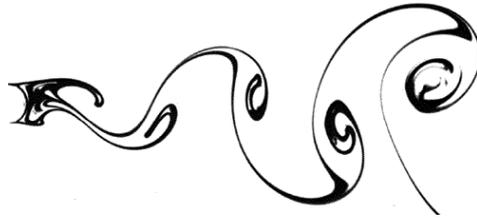
Figure 1.3: Unsteady wake behind a circular cylinder after the first bifurcation.
