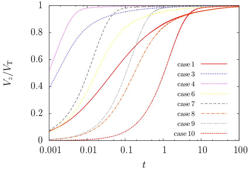
**Figure B.1:** *Falling particle in quiescent fluid: particle velocity time history, Basset force included.*
