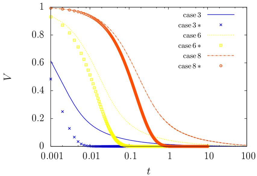
**Figure B.6:** *Particle arresting in quiescent fluid: comparison between the case with and without the Basset History force for cases with  $R = 10$ . Results including the Basset term are displayed by solid lines, results without Basset with symbols.*
