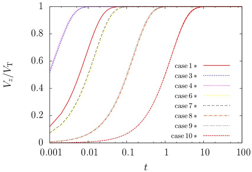
**Figure B.2:** *Falling particle in quiescent fluid: particle velocity time history, Basset force neglected.*
