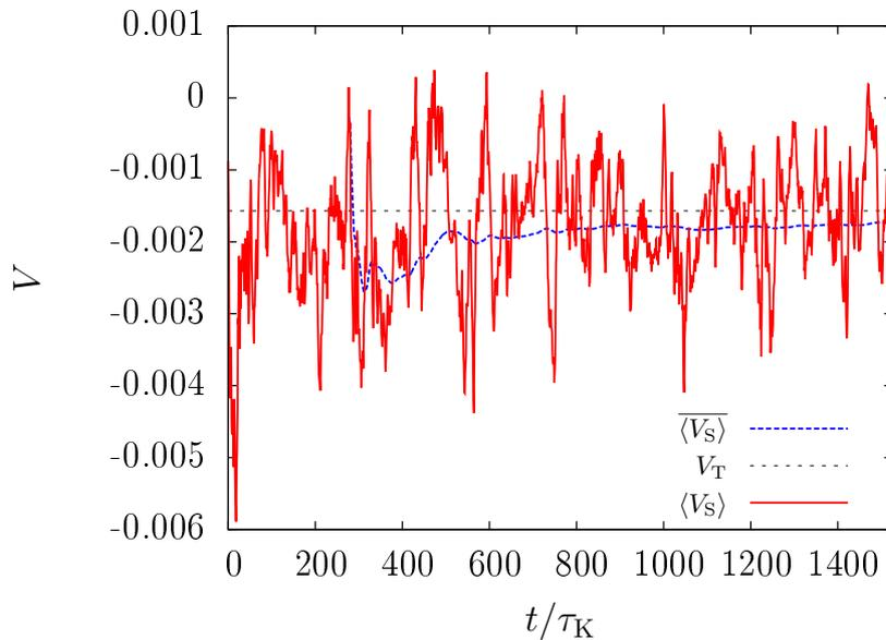
**Figure 6.1:** *Settling velocity, case A. The red curve is the settling velocity averaged over the particles, the blue dashed line its time average, while the black dashed line indicates the theoretical terminal velocity.*
