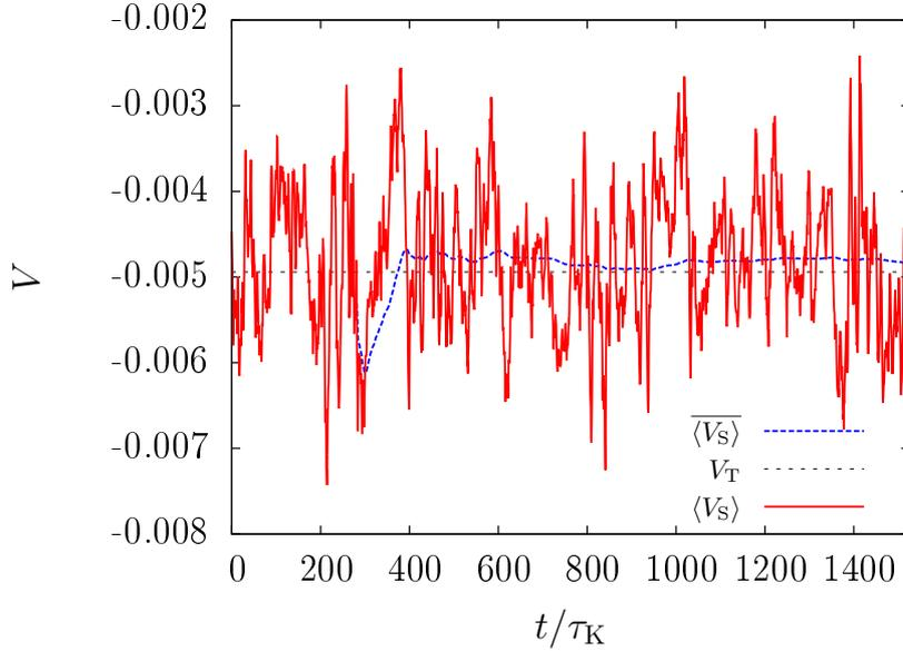
**Figure 6.2:** *Settling velocity, case B. The red curve is the settling velocity averaged over the particles, the blue dashed line its time average, while the black dashed line indicates the theoretical terminal velocity.*
