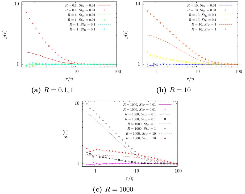
**Figure 5.12:** The radial distribution function  $g(r)$  versus particle distance  $r/\eta$  for different  $R$ . Results including the Basset term are displayed by solid lines, results without Basset with symbols
