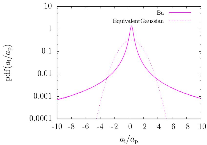
**Figure 5.4:** Comparison between the obtained p.d.f. and the equivalent gaussian distribution with the same mean value and standard deviation, for the Basset curve of case 6 ( $R = 10$ ,  $St_K = 0.1$ ).
