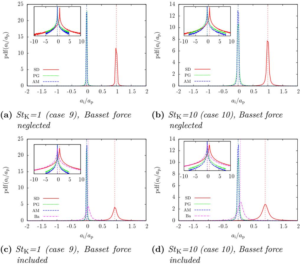
**Figure 5.5:** *P.d.f.'s of the different acceleration ratios  $a_i/a_p$  for particles with  $R = 1000$  (heavy particles). Comparison between simulations with and without the Basset History term computation.*
