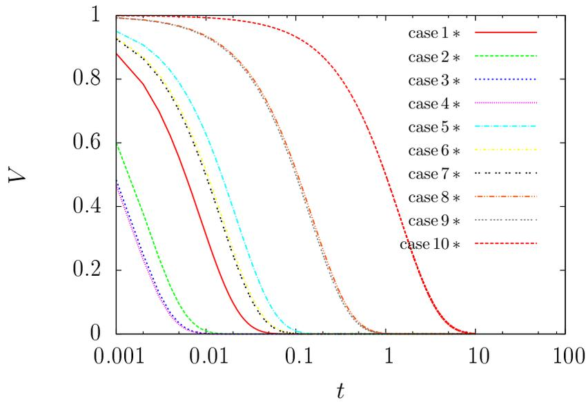
**Figure B.4:** *Particle arresting in quiescent fluid: particle velocity time history, Basset force neglected.*
