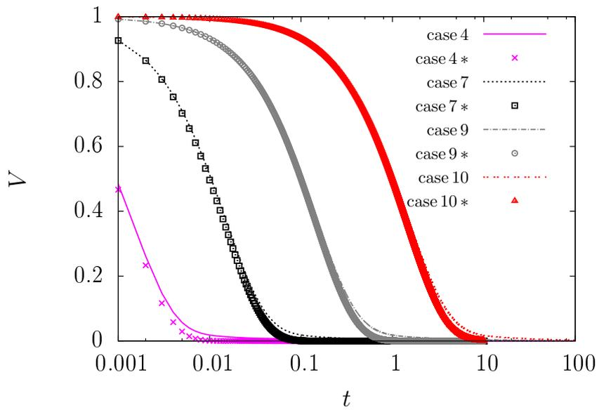
**Figure B.7:** Particle arresting in quiescent fluid: comparison between the case with and without the Basset History force for cases with  $R = 1000$ . Results including the Basset term are displayed by solid lines, results without Basset with symbols.
