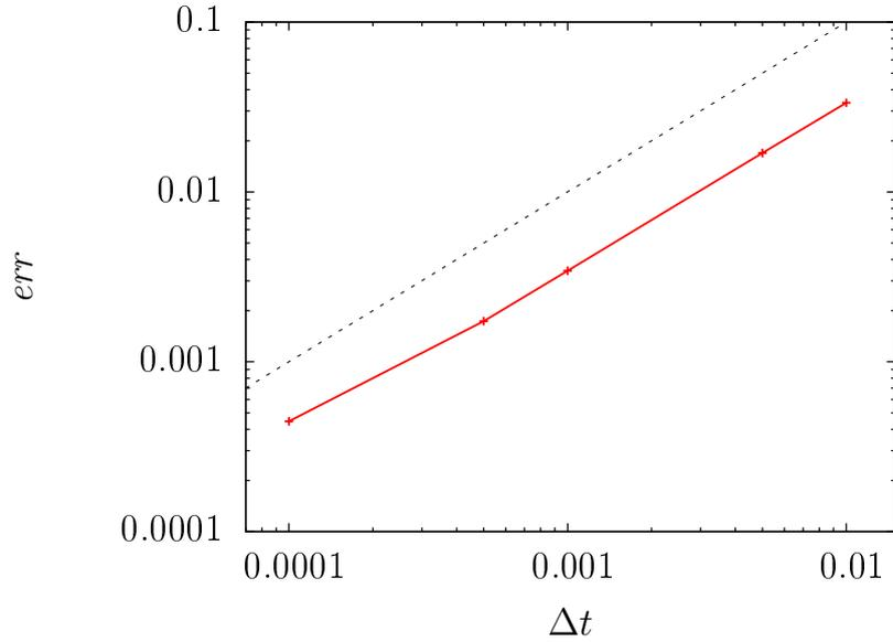
**Figure 3.4:** *Validation Test 1: Relative error as a function of the simulation time step. Red points are the results of the code while the black dashed line represents a first order slope.*
