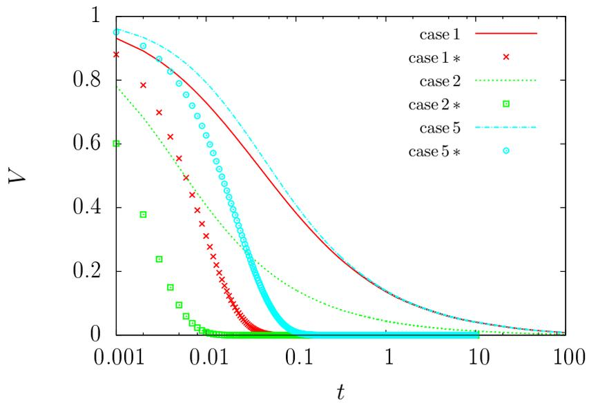
**Figure B.5:** *Particle arresting in quiescent fluid: comparison between the case with and without the Basset History force for cases with  $R = 0.1, 1$ . Results including the Basset term are displayed by solid lines, results without Basset with symbols.*
