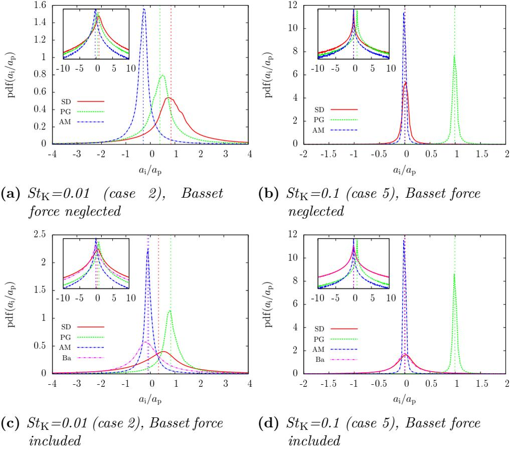
**Figure 5.6:** *P.d.f.'s of the different acceleration ratios  $a_i/a_p$  for particles with  $R = 1$  (neutrally-buoyant particles). Comparison between simulations with and without the Basset History term computation.*
