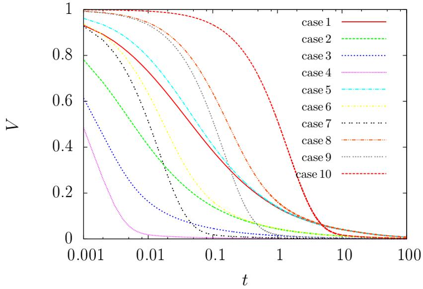
**Figure B.3:** *Particle arresting in quiescent fluid: particle velocity time history, Basset force included.*
