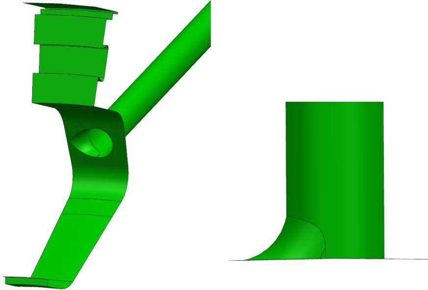
*Fig. 3.7: Front view (left) and  $x - \theta$  view (right) of the RB fillet inlet.*
