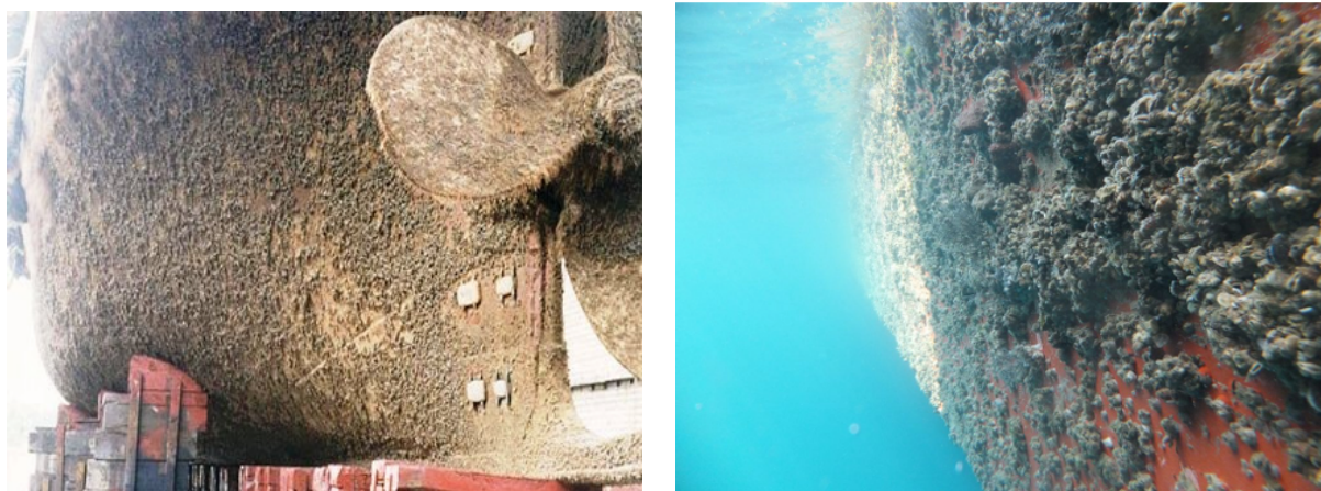
Figure 1.4: Pictures of biofouling impact on the hull of a vessel.
