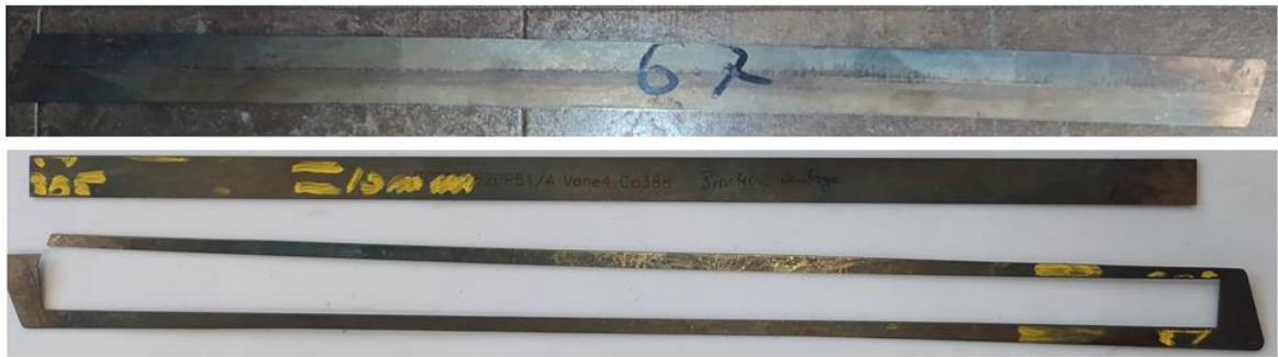
Figure 3.14 – example of upgrade-thin strip seal – worn
