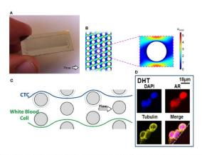
FIGURE 2 | Geometrically-enhanced differential immunocapture (GEDI) microfluidic device. (A) GEDI Chip (B) GEDI post-array (C) illustration of laminar flow through GEDI device (D) Captured CTCs stained for AR and tubulin.
