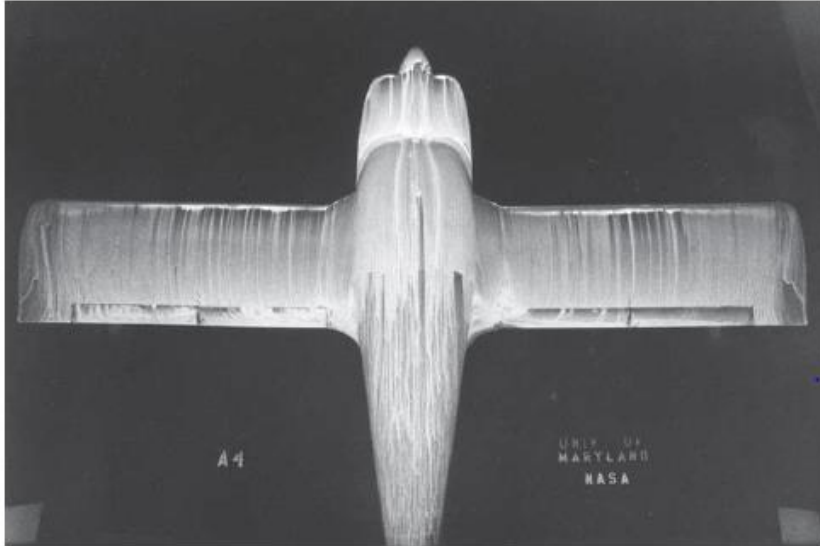
Below stall – Flow attached
