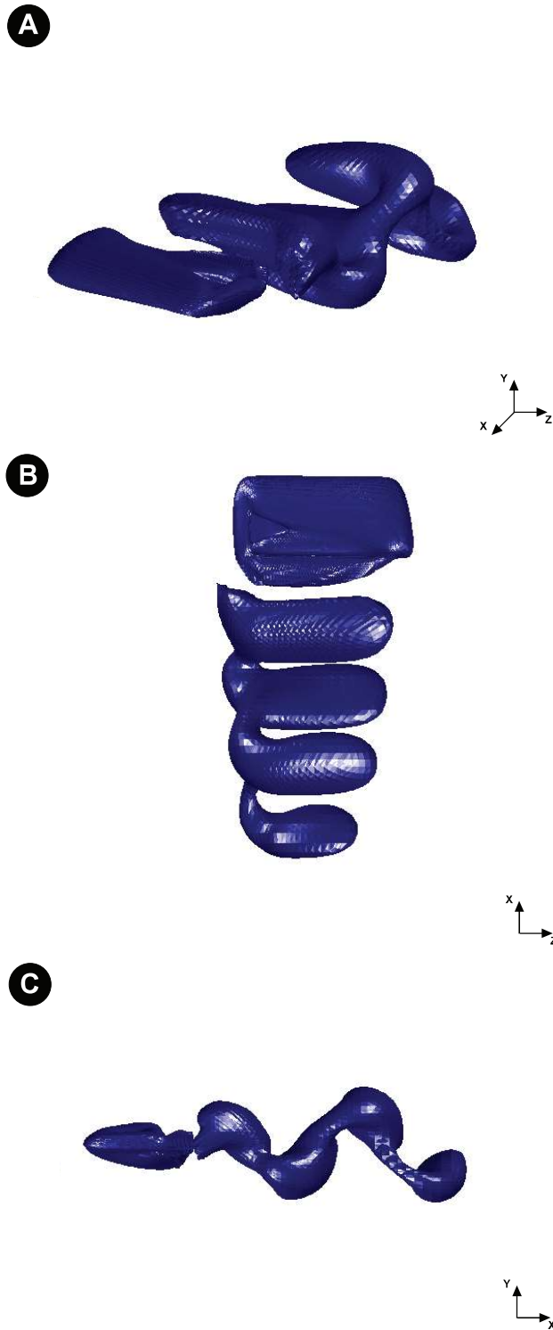
Figure 8.19: Vortex topology for the rolling wing case ( t=5.0 ). Flapping parameters: St = 0.10 , f_{roll} = 1.0 , Re = 500 . A) Perspective view. B) Top view. In this view the right wing-tip corresponds to the hinged extreme. C) Side view.
