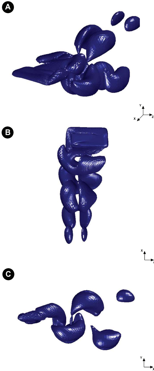
Figure 8.20: Vortex topology for the rolling wing case ( t=5.0 ). Flapping parameters: St = 0.25 , f_{roll} = 1.0 , Re = 500 . A) Perspective view. B) Top view. In this view the right wing-tip corresponds to the hinged extreme. C) Side view.
