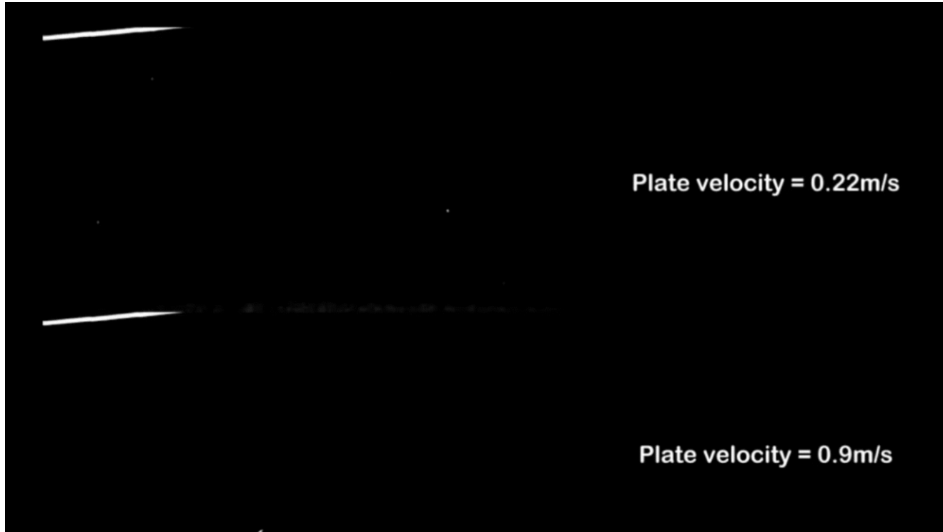
Turbulent boundary layer on a flat plate
