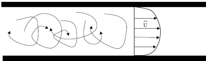
Turbulent flow in a channel or pipe
