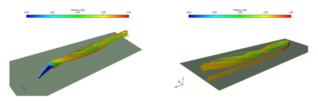
Streamlines released from the vane – Colored using pressure field
