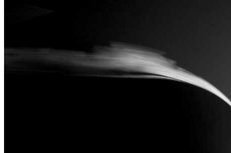
(e) Smoke visualisation of separation over top
