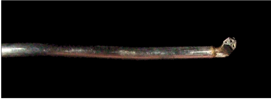
Figure 2.9: Detail of Series 100 TFI Cobra Probe
