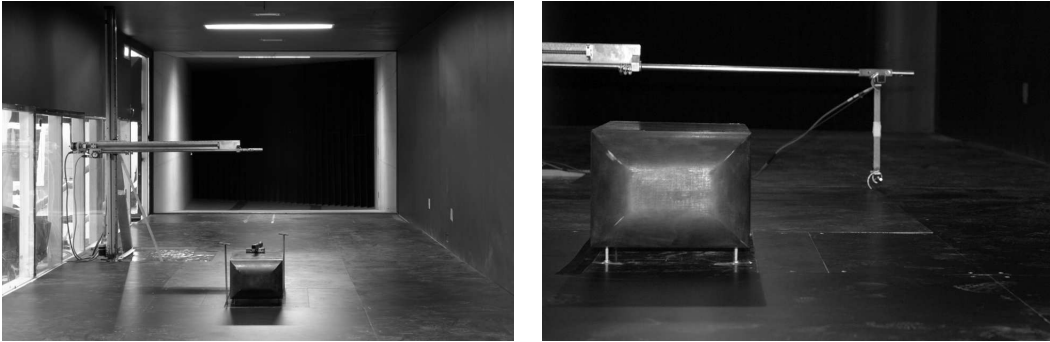
Figure 2.12: RMIT three-axis traverse during pre-fit
