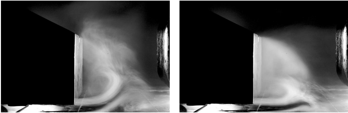
Figure 4.22: Underbody flows about base of leading model in \alpha = 25/25^\circ platoon, \frac{x}{L} = 0.25 spacing
