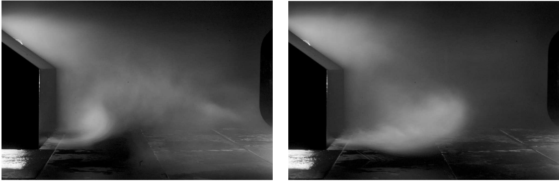
Figure 4.28: Underbody flows about base of leading model in \alpha = 35/25^\circ platoon, \frac{x}{L} = 0.5 spacing
