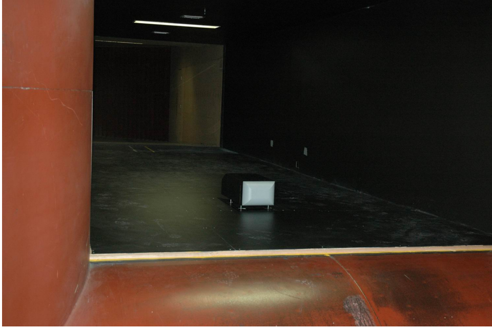
Figure 2.4: Ahmed Model installed in test section
