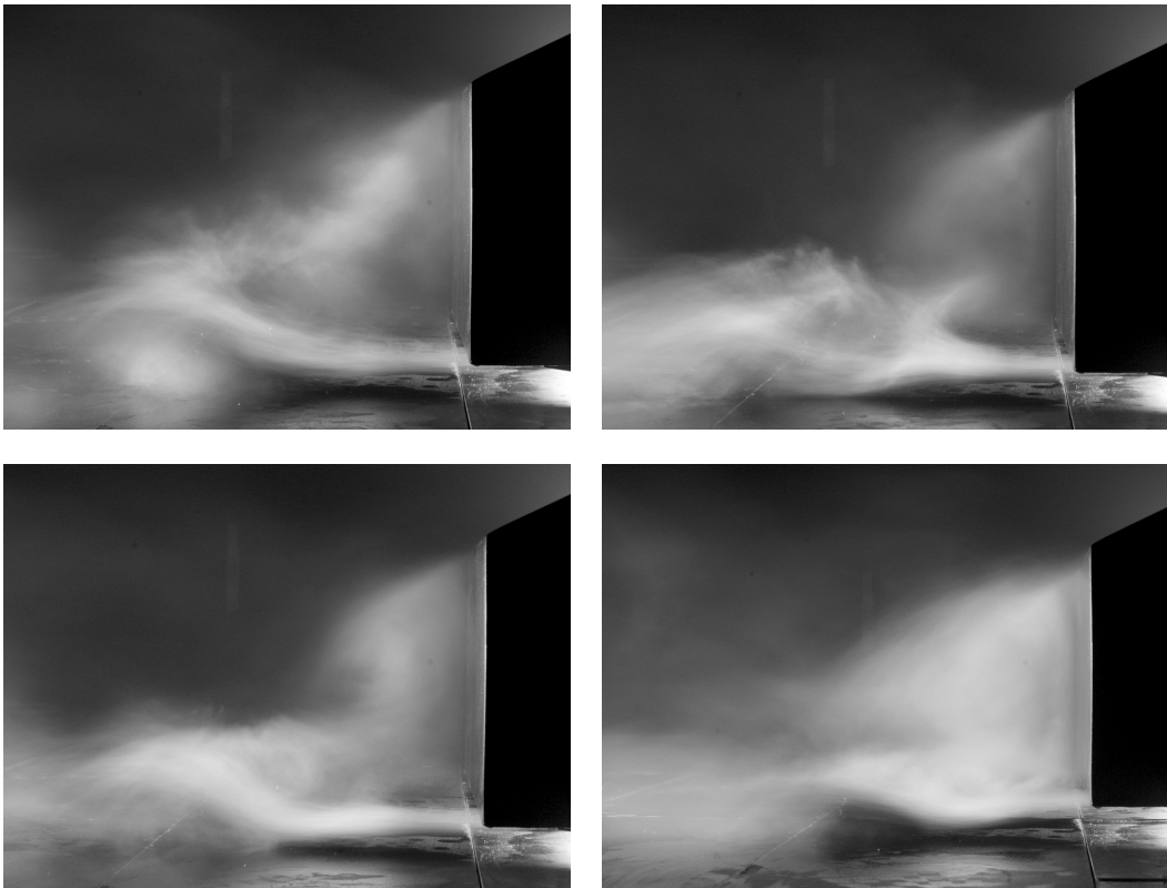
Figure 3.29: Shedding at base of \alpha = 25^\circ Ahmed model
