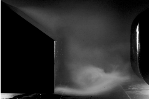
(b) Underbody flows about base of leading model
