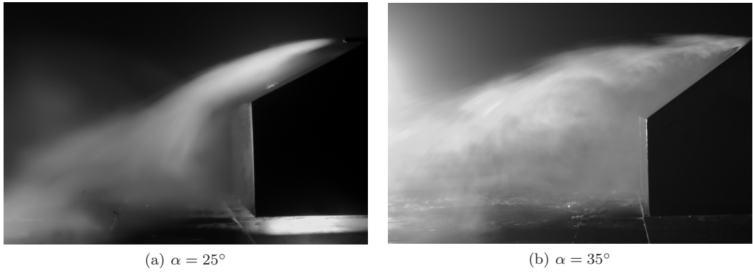
Figure 3.6: Smoke injected over backlight at centreline
