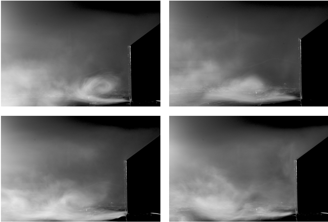
Figure 3.32: Shedding at base of \alpha = 35^\circ Ahmed model
