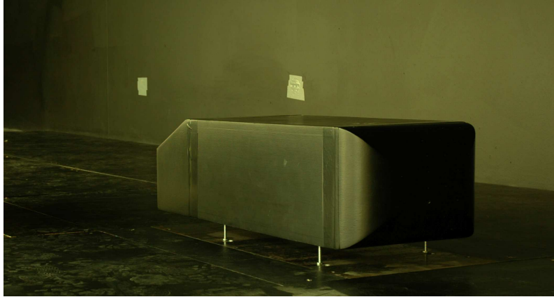
Figure 2.1: Single Ahmed Model installed in RMIT IWT
