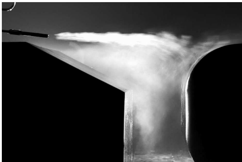
Figure 4.16: Centreline impingement on second model in \alpha = 25/25^\circ platoon, \frac{x}{L} = 0.125 spacing
