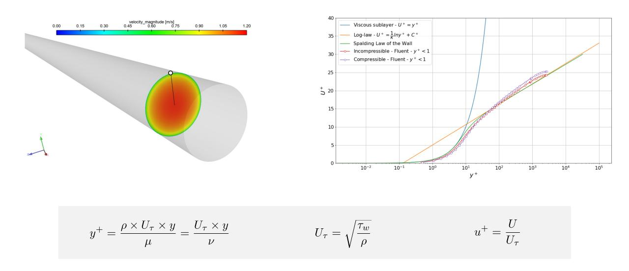
To do the plot of u<sup>+</sup> vs. y<sup>+</sup>, you will need to sample wall shear stress and velocity in a location where the flow is fully developed and there is no separation.
