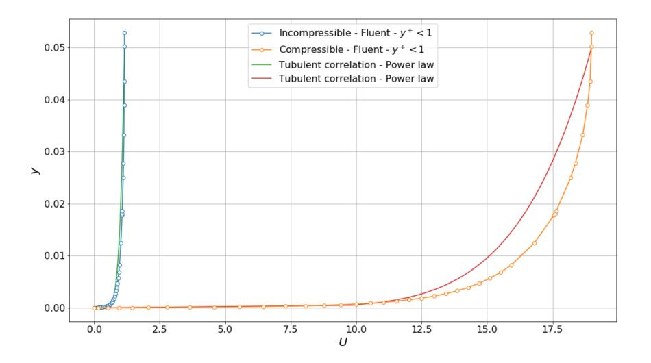
• Comparison of the velocity profiles in the turbulent regime – Comparison of incompressible and compressible case.
