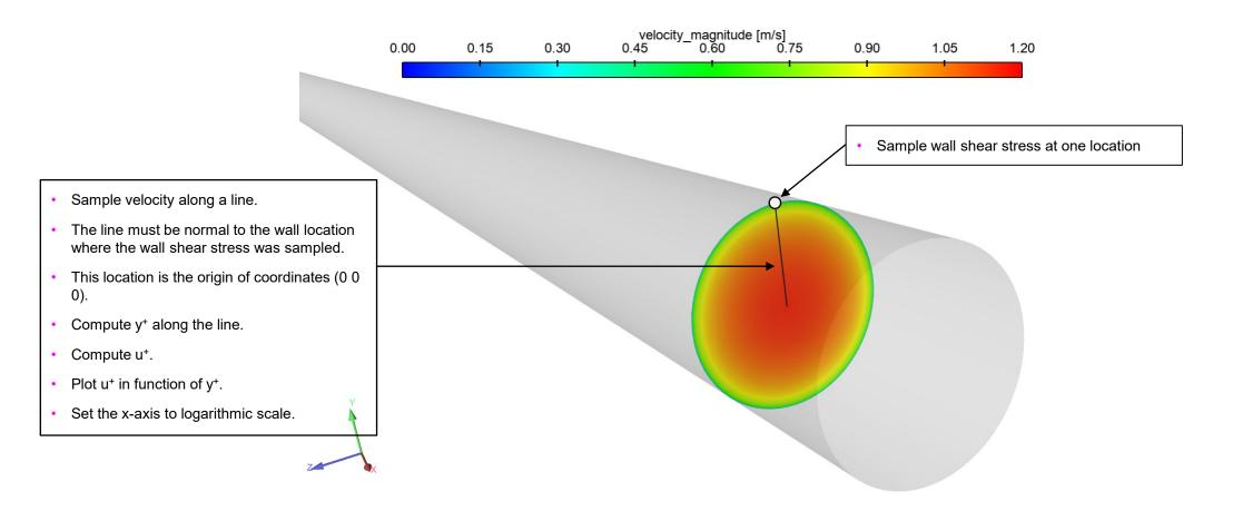
To do the plot of u<sup>+</sup> vs. y<sup>+</sup>, you will need to sample wall shear stress and velocity in a location where the flow is fully developed and there is no separation.
