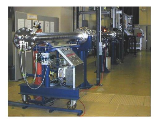
Shock tube. The driver section, including vacuum pumps, controls, and helium driver gas. Photo credit: Stanford University. http://hanson.stanford.edu/index.php?loc=facilities\_nasa
