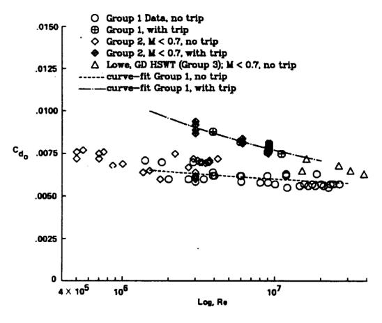
Fig. 4. Drag coefficient at zero lift vs. Reynolds number.
