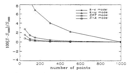
Figure 5. Comparison of spreading rate sensitivity to grid resolution for compressible mixing layer.
