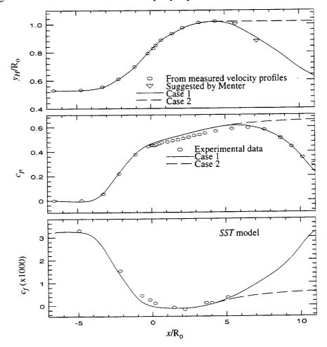
Figure 14.7. Effects of position of the outer streamline in the outflow region.
