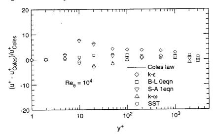
Figure 12.12. Percentage errors with respect to Coles' velocity profile— $Re_{\theta} = 10^4$ .
