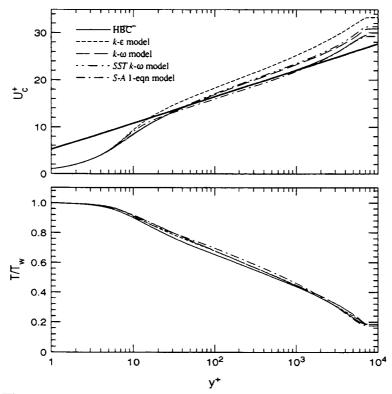
Figure 13.2. Comparison of velocity and temperature profiles.
