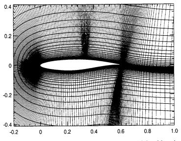
Figure 16.1. Computational grid with  $386 \times 82$  points.
