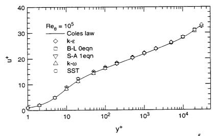
Figure 12.11. Comparison of the velocity profiles— $Re_{\theta} = 10^5$ .
