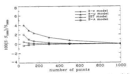
Figure 8.3. Comparison of spreading rate sensitivity to grid resolution for plane jet flow.
