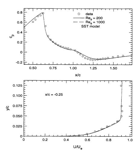
Figure 15.6. Effects of inlet boundary layer profiles.
