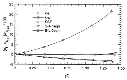
Figure 12.2. Sensitivity to the distance of the first point to the wall.
