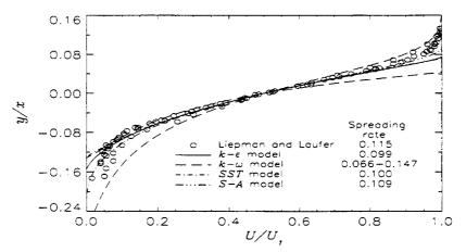
Figure 7.1. Comparison of velocity profiles for mixing layer flow.
