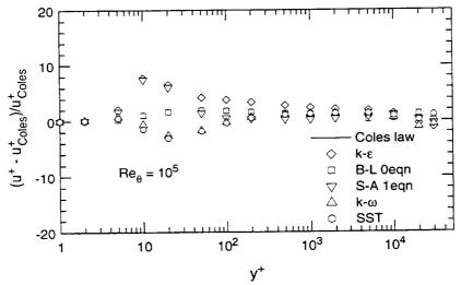
Figure 12.13. Percentage errors with respect to Coles' velocity profile— $Re_{\theta} = 10^5$ .
