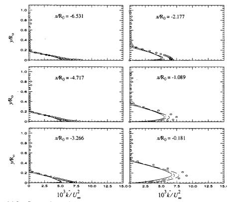
Figure 14.3a. Comparison of the turbulent-kinetic energy profiles. See symbols in figure 14.1.
