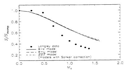
Figure 11.3a. Comparison of spreading rate of the mean velocity profile for compressible mixing layer.
