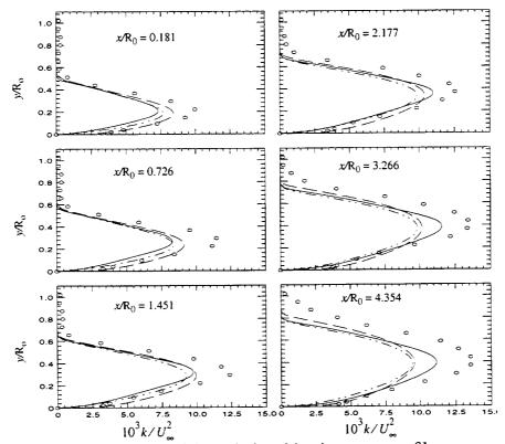
Figure 14.3b. Comparison of the turbulent-kinetic energy profiles.
