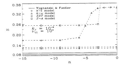
Figure 9.2. Comparison of spreading rate sensitivity to freestream turbulence for round jet flow.
