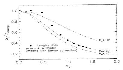
Figure 11.3b. Comparison of spreading rate of the mean velocity profile for compressible mixing layer.
