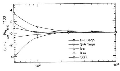
number of points Figure 12.1. Grid sensitivity study—flat plate boundary layer.
