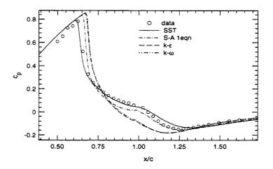
Figure 15.1. Comparison of surface pressure coefficient—transonic bump flow.
