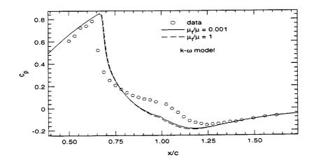
Figure 15.7. Effects of freestream conditions for the k- $\omega$  model.
