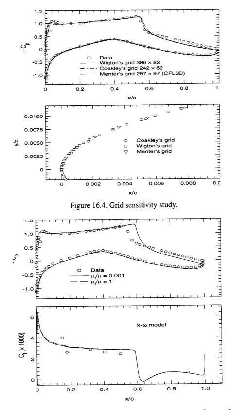
Figure 16.5. Effects of freestream boundary conditions on the k- $\omega$  model.
