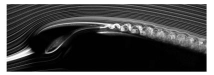
Flow around an airfoil with a leading-edge slat Photo credit: S. Makiya et al.
