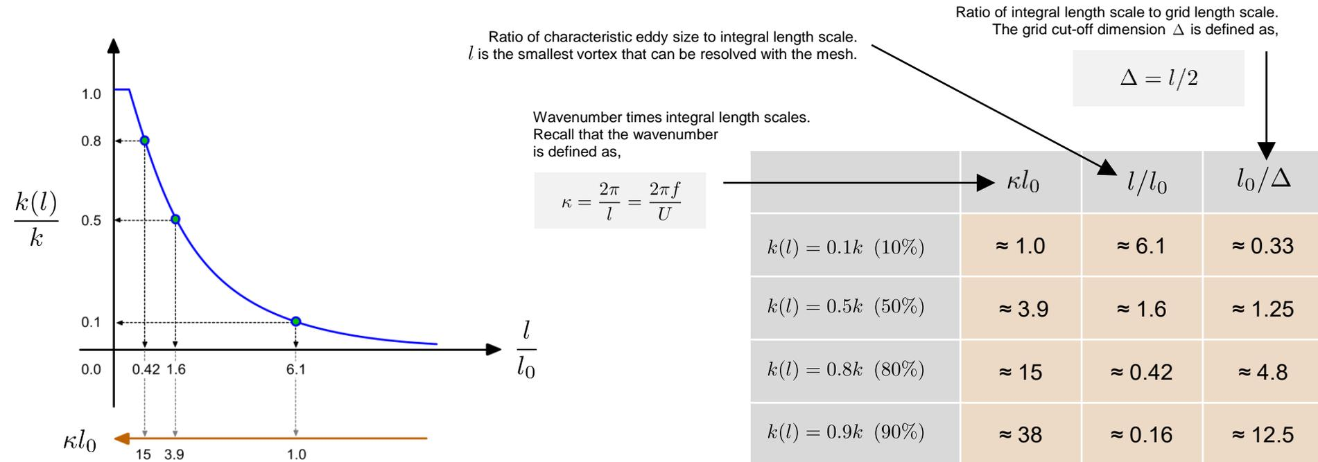
Cumulative turbulent kinetic energy plot against lengths scale of eddies for a model spectrum function. The figure has been adapted from reference [1].
