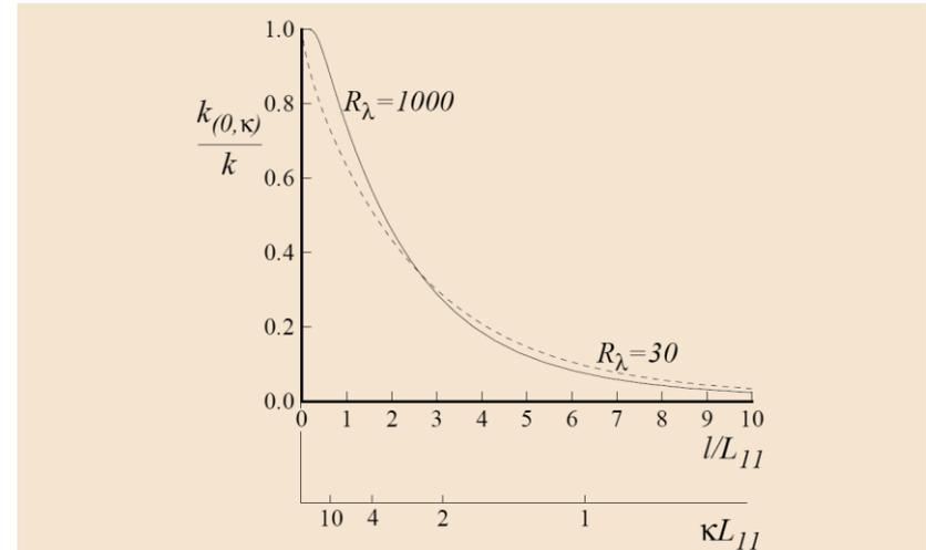
Cumulative turbulent kinetic energy against wavenumber and wavelength for a model spectrum [1].
