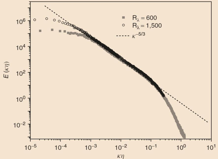
Experimental spectra measured in the boundary layer of the NASA Ames 80 x 100 foot wind tunnel [2].
