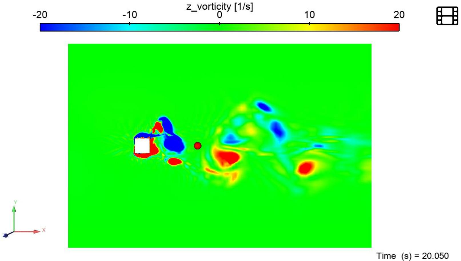
**Vorticity contours – The velocity field is being sampled at the red sphere.**
