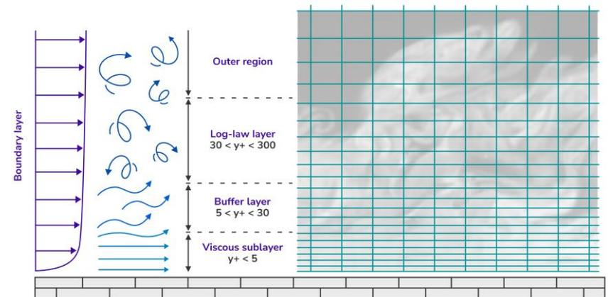
Resolving the streamwise direction is also important, for example, when dealing with transition to turbulence.
