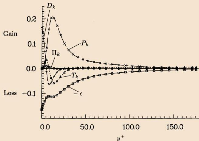
Figure 5. Terms in the budget of the turbulence kinetic energy,  $k$ , in wall coordinates.  $P_k$  = Production;  $T_k$  = Turbulent transport;  $D_k$  = Viscous diffusion;  $\epsilon_k$  = Dissipation rate;  $\Pi_k$  = Velocity pressure-gradient term.
