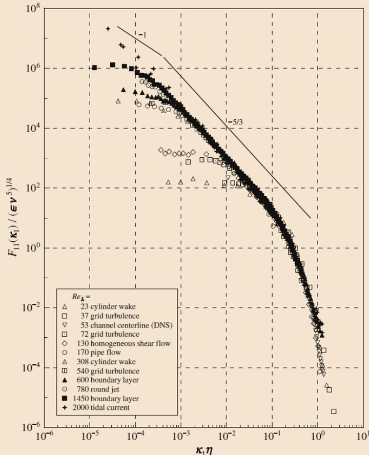
One-dimensional spectra scaled with respect to the microstructure from various turbulent flows. This demonstrates the universal character of the microstructure and illustrates the  $-5/3$  behavior of the inertial subrange [1].
