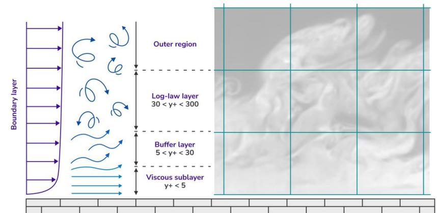
Insensitive wall treatment will automatically switch between the wall modeling approach or the wall resolving approach according to the  $y^+$  value.
