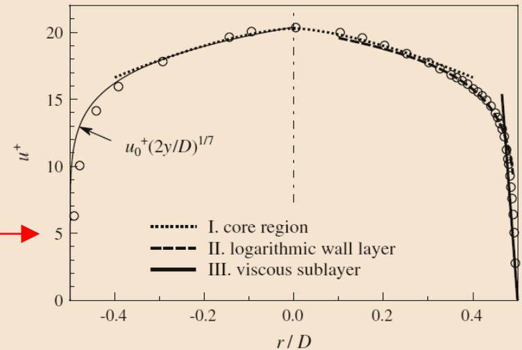
The dimensionless mean velocity profile  $u^+$  of a turbulent flow in a pipe at  $Re = 10000$  as a function of the distance  $r$  from the centerline of a pipe with diameter  $D$ , compared to experimental data.
