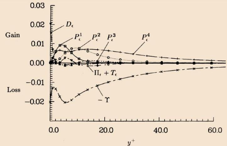
Figure 6. Terms in the budget of the dissipation rate of the turbulence kinetic energy,  $\epsilon$ , in wall coordinates.  $P_\epsilon^1$  = Production by mean velocity gradient;  $P_\epsilon^2$  = Mixed production;  $P_\epsilon^3$  = Gradient production;  $P_\epsilon^4$  = Turbulent production;  $T_\epsilon$  = Turbulent transport;  $D_\epsilon$  = Viscous diffusion;  $\Upsilon$  = Dissipation rate;  $\Pi_\epsilon$  = Pressure transport.
