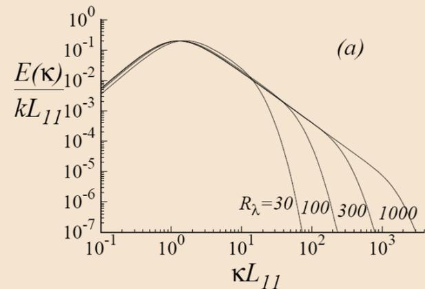
The model spectrum for various Reynolds number scaled by  $k$  and  $L_{11}$  [1].
