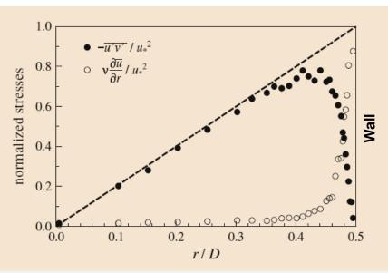
The total normalized stress (using wall shear stress), as a function of the distance r from the centerline of a pipe with diameter D. The total stress consists of a contribution from the Reynolds stress (black circles) and the viscous stress (empty circles). Experimental data for a turbulent pipe flow at Re = 10000 [1].
