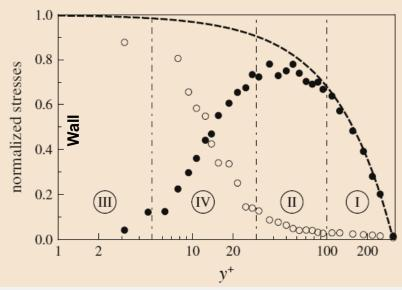
The same data as in the left figure, but now as a function of the dimensionless distance  $y^+$  from the pipe wall in a semi-log plot. In the figure, I = core region; II = logarithmic wall region; III = viscous sublayer; IV = buffer layer. Note that r = 0 corresponds to  $y^+ = 312$  and r = 0.5D to  $y^+ = 0$  [1].
