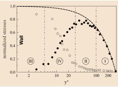
The same data as in the left figure, but now as a function of the dimensionless distance  $y^+$  from the pipe wall in a semi-log plot. In the figure, I = core region; II = logarithmic wall region; III = viscous sublayer; IV = buffer layer. Note that r = 0 corresponds to  $y^+ = 312$  and r = 0.5D to  $y^+ = 0$  [1].
