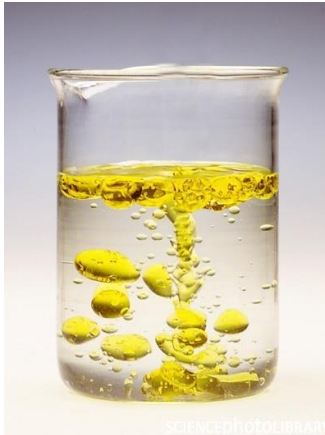
Water + oil = multiphase Clear and distinct interface
