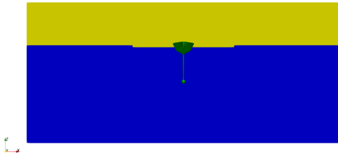
Non-uniform cell size at the interface
