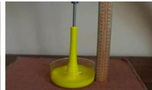
Visco-elastic fluids – Weissenberg effect. Dough tend to climb up rotating shafts
