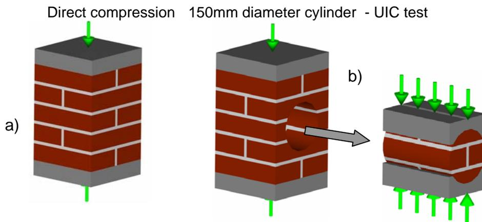
Figure 3. Identical specimens for: a) direct concentric compression; b) UIC (1995) tests.
