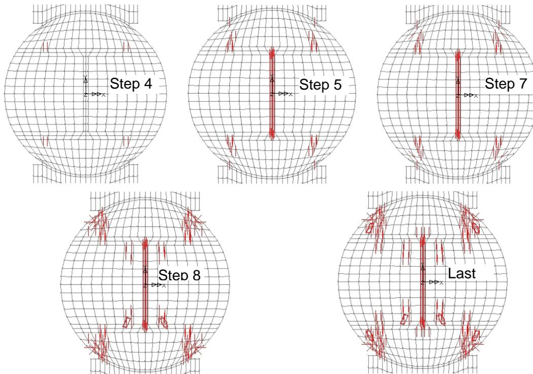
**Figure 9.** Crack pattern evolution during the load process
