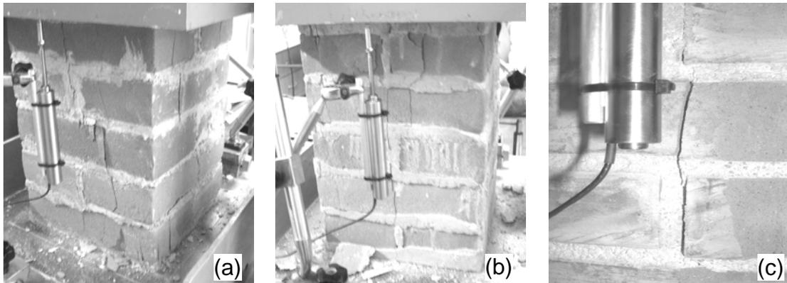
**Figure 7.** BRICKWORK 1 and 2: cracking of prisms at approx. 80% of the peak load.
