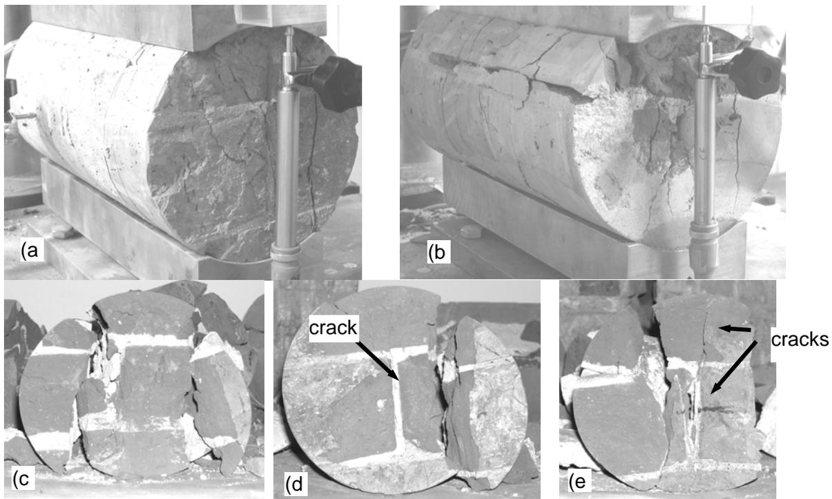
**Figure 5.** BRICKWORK 1 and 2: typical crack pattern at: a) 80% of the maximum load; b) end of the test; c), d) and e) typical collapse mechanisms: opening of the vertical joint and splitting of the lateral part of the cylinder (after peak load).
