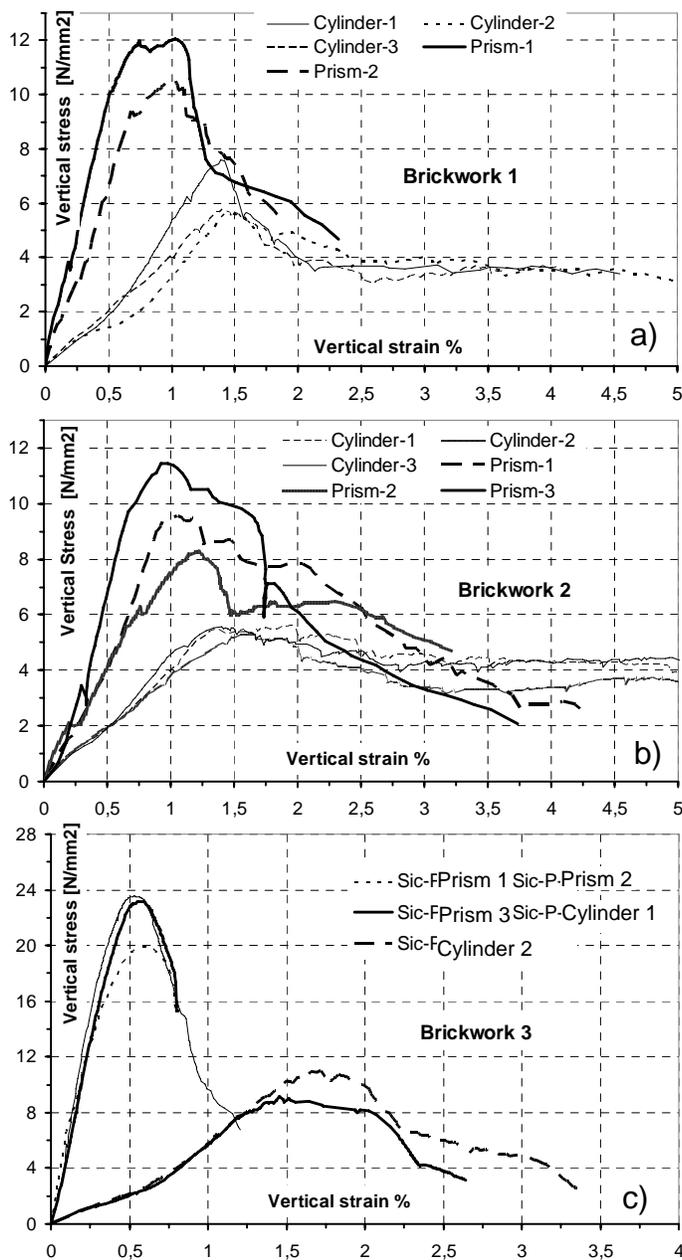
**Figure 4.** Stress-strain curves for brickwork.
