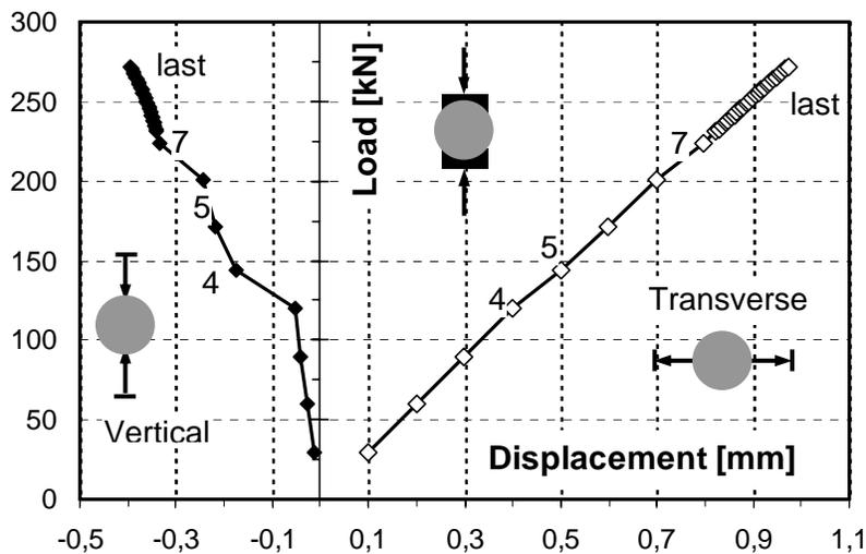
**Figure 8.** Load-displacement response of the FEM model.
