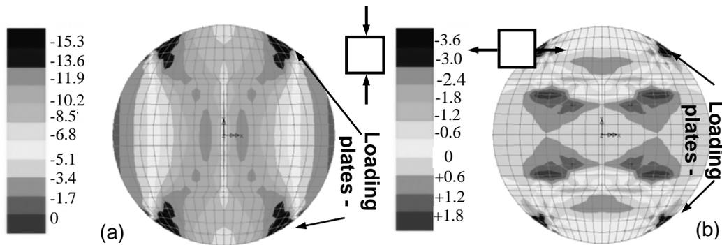
**Figure 10.** a) Vertical and b) horizontal stresses [MPa], 80% of peak load
