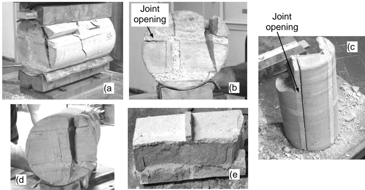
**Figure 6.** BRICKWORK 3: typical crack pattern at the maximum load. Cyl. 1: a) the lateral parts detach and b) the brick/mortar interface collapses before collapse is activated; c) detachment of the joint. Cyl. 2: d) the same collapse mechanism as for Cyl. 1; e) detachment of the horizontal joints.
