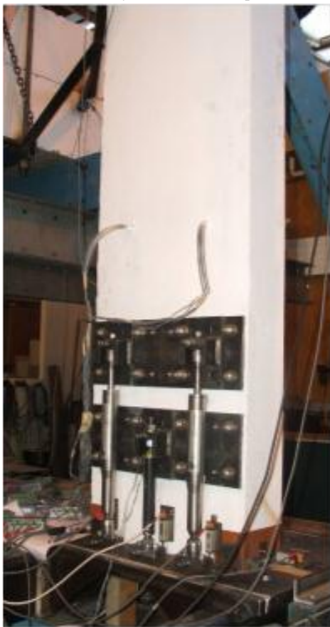
Figure 20: Concept, implementation and experimental validation (shake-table) of the concept of Advanced Flag-Shape applied to a post-tensioned wall (Kam et al. , 2010; Marriott et al. , 2008). Combination in parallel of hysteretic and viscous dampers.
