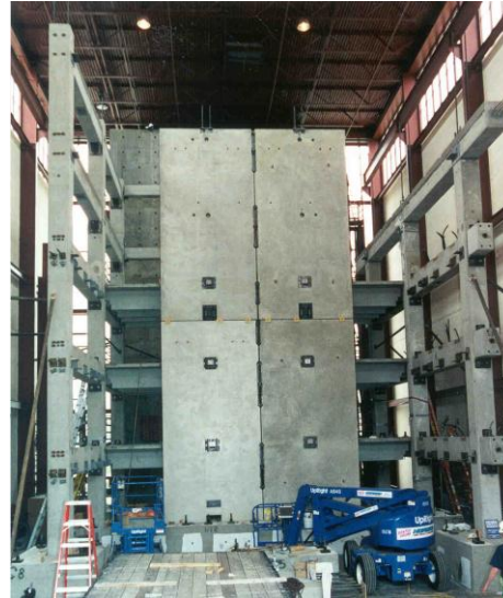
Figure 9: Five-Storey PRESSS Building tested at University of California, San Diego (Priestley et al. , 1999).
