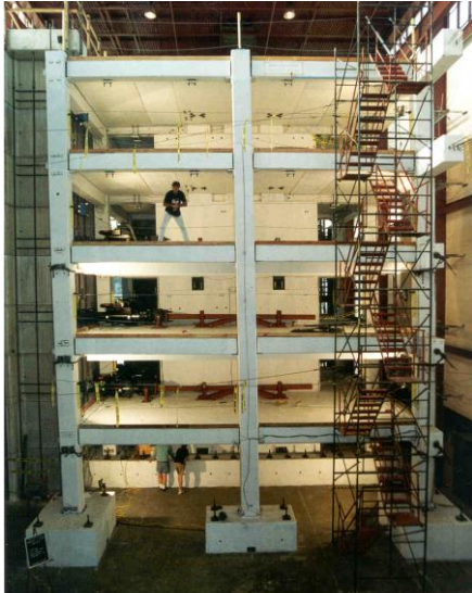
Figure 9: Five-Storey PRESSS Building tested at University of California, San Diego (Priestley et al. , 1999).
