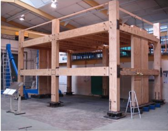
Figure 34: From laboratory specimen to office building: 3D Test Specimen tested in the lab (Newcombe et al, 2010), dismantled and reconstructed (Smith et al., 2011) on UC campus as EXPAN/STIC office.
