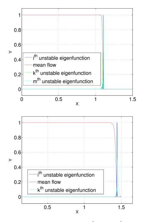
Figure 11: All unstable eigenfunctions for  $\tilde{A} = 0.4$  and  $\tilde{A} = 1$  with  $\Delta_x = 10^{-3}$  and  $\theta = \pi/24$ . (For  $\tilde{A} = 5$  and  $\tilde{A} = 10$  there is only one unstable eigenfunction).
