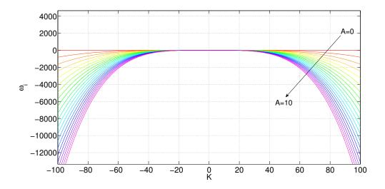
Figure 7: Analytical solution for  $Im(\omega)$ . No unstable modes can be seen.
