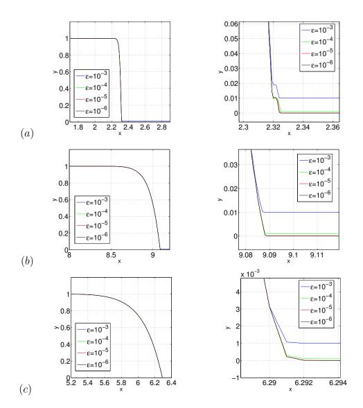
Figure 4: Steady solution for varying thickness  $\epsilon$  of the precursor film, with  $\Delta_x = 10^{-3}, \Delta_t = 10^{-2}, \tilde{A} = 1$  (frame (a)),  $\tilde{A} = 5$  (frame (b)) and  $\tilde{A} = 10$  (frame (c)), after 30000 steps in time.
