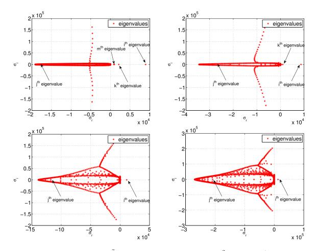
Figure 8: Spectrum of  $\Omega$  for  $\tilde{A} = 0.4, 1, 5, 10$  with  $\Delta_x = 10^{-3}$  and  $\theta = \pi/24$ .
