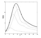
Figure : Amplification G(t) for Poiseuille flow with Re = 1000,  $\alpha = 1$ (solid line) and growth curves of selected initial conditions (dashed lines). The quantity G(t) gives the maximum amplification optimized over all possible initial conditions. In general, each point on the curve G(t) is arrived at by a different initial condition, and G(t) represents the envelope of individual growth curves, see figure.
