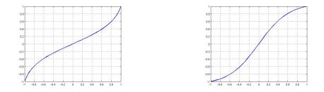
Both profiles lead to unstable solutions according to Rayleigh's criterion; however the inflection point has to be a maximum of the spanwise vorticity (not a minimum).
