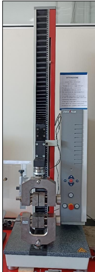
Figure 46: Zwick Roell BL-GRS010K 10kN
