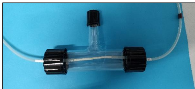
Figure 35: Prosthesis inserted in the home-made bioreactor chamber
