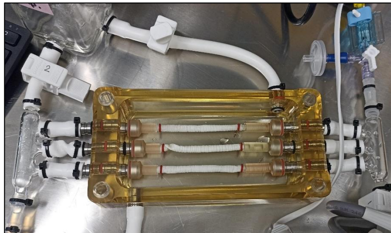
Figure 36: Prosthesis inserted in the chamber of the high-performance bioreactor
