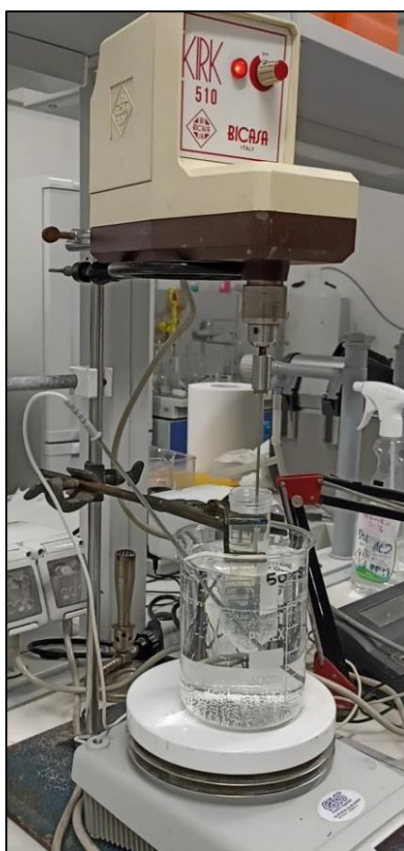
Figure 29: Prostheses were submerged into the gelatine-based solution, placed on a mechanical stirrer
