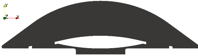
Figure 6.5: Cross section of the anterior chamber with aIOL and system of coordinates.
