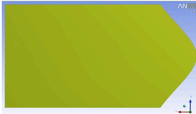
FIGURE 7.2. Domain C around the airfoil. The length of the rectangular is 150 meters, the high 90 meters and the chord of the airfoil is 1 meter.
