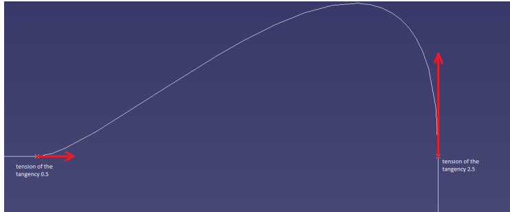
FIGURE 4.2. Effects of different tensions of a spline near to two fixed control points.
