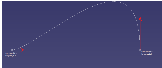
FIGURE 6.3. Example of different values of tension of the spline near two fixed control points.
