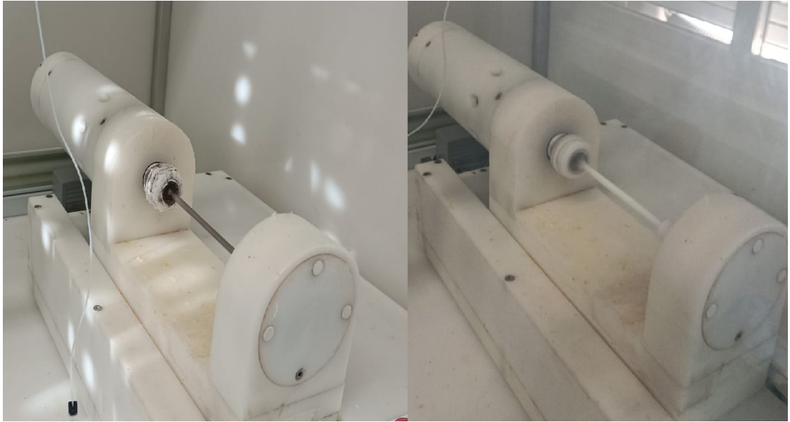
Figure 6.3: Electrospinning machine used for sample production. On the left, the machine is idle before production. On the right, the machine is in operation, halfway through the sample production process.
