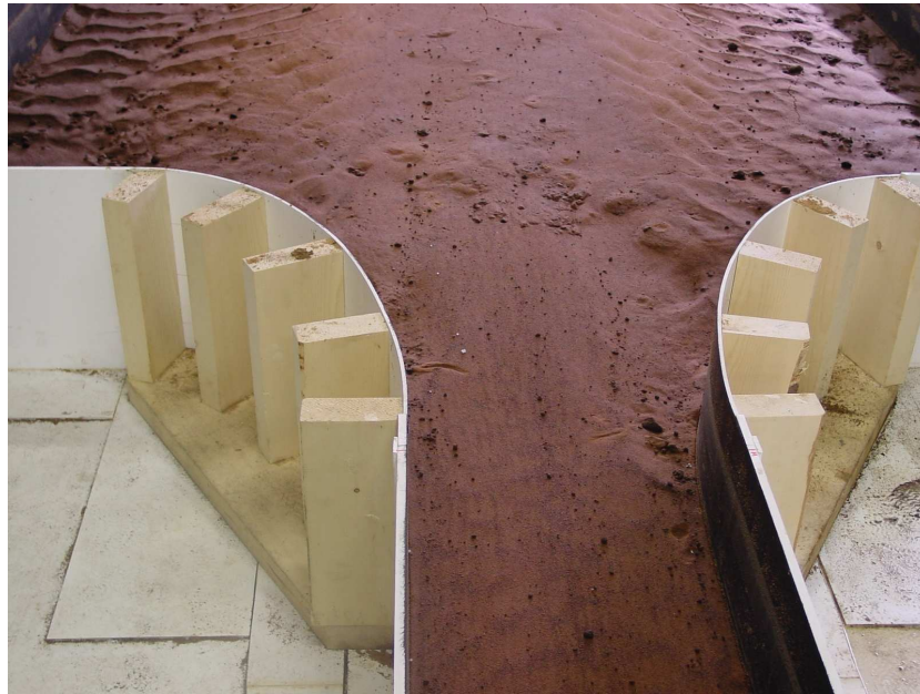
Figure 3.6: The smooth shape of the inlet walls in the second experiment.
