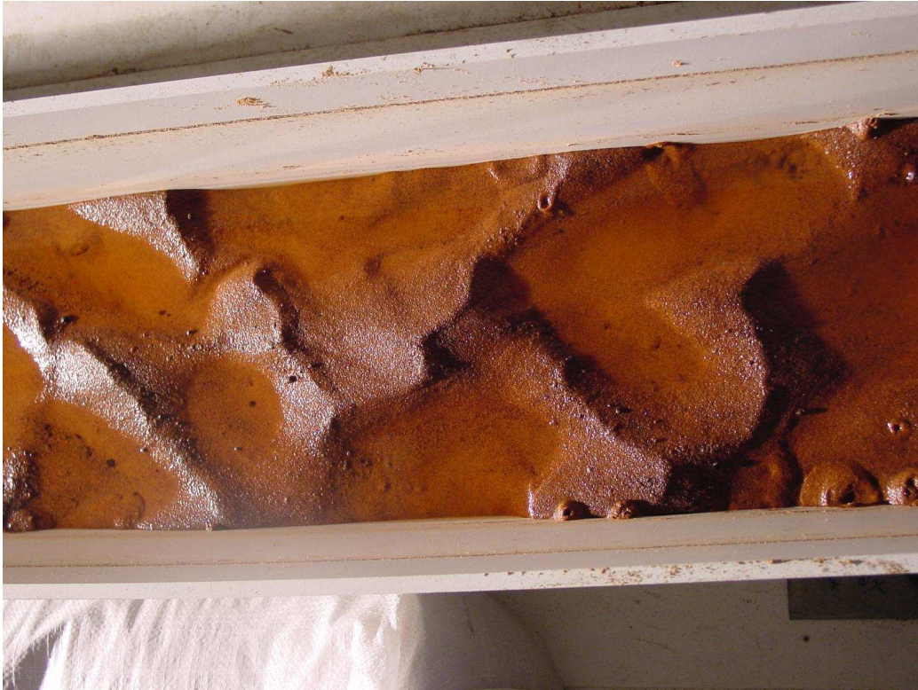
Figure 3.34: A picture of the complex 3D ripple pattern observed in the second experiment.
