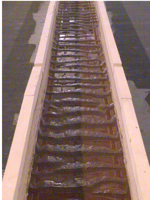
Figure 3.18: A picture of the ripple pattern observed along the channel in the initial phase of experiment 1.
