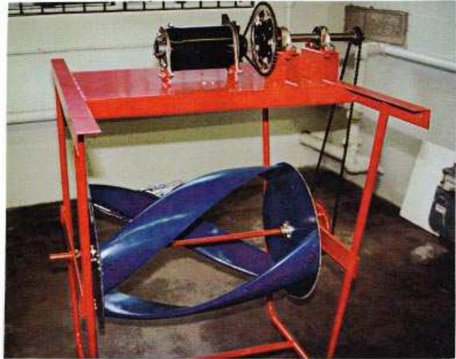
*Fig. 2.32 - Double and triple helical turbine (Lucid energy technologies).*
