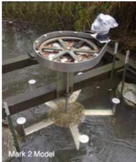
*Fig. 2.29 - Darrieus turbine (Alternative Hydro Solutions Ltd).*
