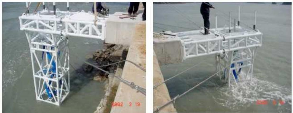
*Fig. 2.36 - Twin Triple-helix GHT in the Uldolmok Strait (Lucid energy technologies).*
