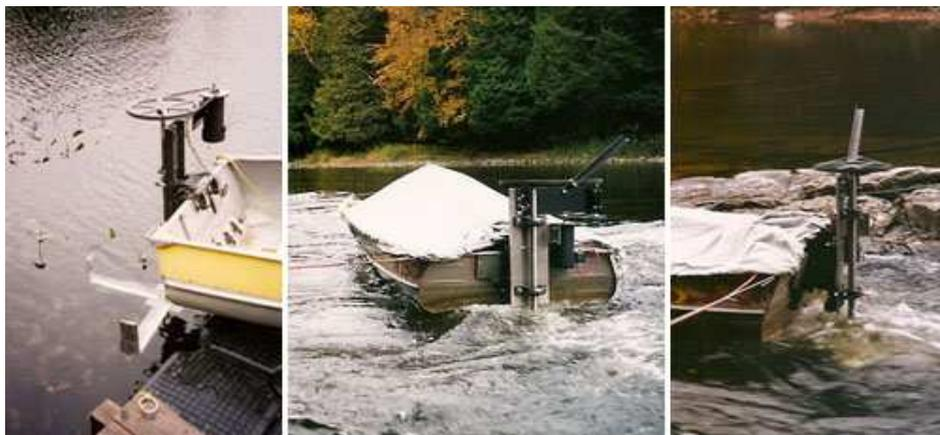
Fig. 2.31 - Mounting schemes for Darrieus turbine (Alternative Hydro Solutions Ltd).
