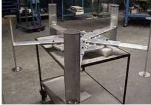
*Fig. 2.28 - Darrieus turbine rotor and blades (Alternative Hydro Solutions Ltd).*
