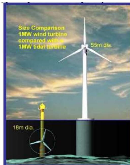
Fig. 2.15 - Size comparison of a 1 MW wind and tidal turbine ( Marine Current Turbines Ltd.).
