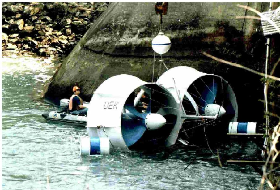
*Fig. 2.21 - UEK Twin Turbines prepared for demonstration (Underwater Electric Kite).*
