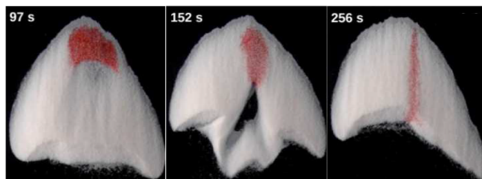
Figure 1: Spreading of grains from an impacting barchan over the target one during the first stage of the diffusion-like mechanism (Assis and Franklin, submitted).
