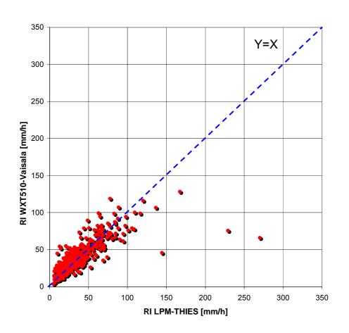
Apart few outliers, the experimental points in the comparison plots show reasonably similar behaviour. It means that the measuring principle adopted by the optical and impact disdrometers gives comparable results with respect to the reference RI, though the manufacturer's calibration procedures are totally different.
