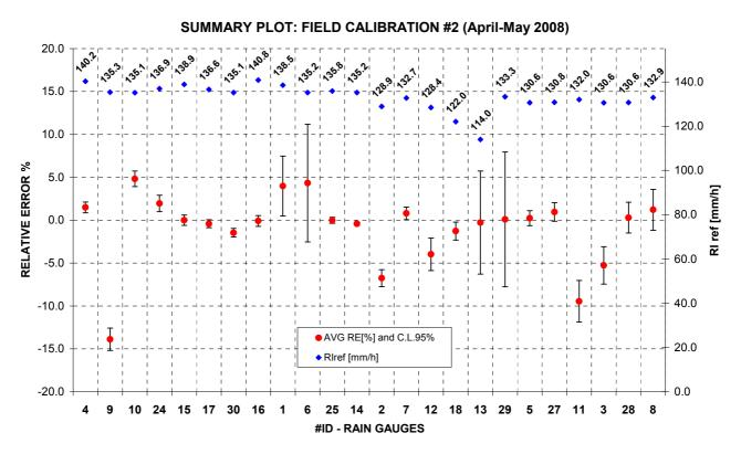
**Fig. 26:** The second field calibration (Vigna di Valle, Italy). The orange dots are the rain gauges relative errors with respect to the reference and whisker caps represents the 95% confidence level interval. Blue dots represent the reference RI generated during the field calibration
