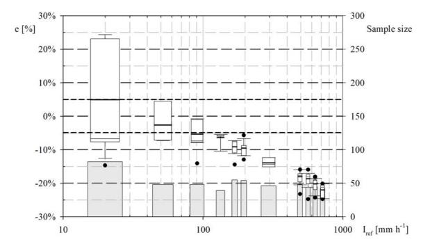
**Fig. 19**: One-minute variability for a sample not corrected TBRG observed performance and the size of the sample used for calculation of the statistics at each reference intensity.
