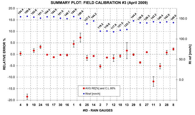
**Fig. 27:** The third field calibration (Vigna di Valle, Italy). The orange dots are the rain gauges relative errors with respect to the reference and whisker caps represents the 95% confidence level interval. Blue dots represent the reference RI generated during the field calibration. Here the #29 is the PLUVIO-OTT.
