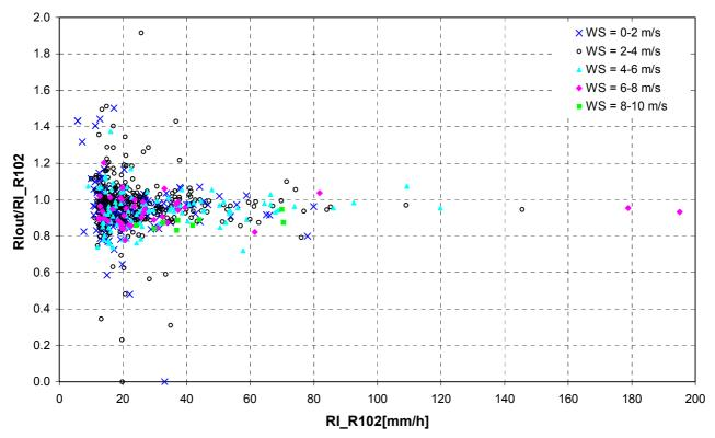
Fig. 48: 1-min R102-ETG RI; RI<sub>out</sub>/RI<sub>pit</sub> vs RI<sub>pit</sub> is shown, divided in groups of wind speed conditions.
