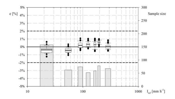
Fig. 18 One-minute variability for a sample corrected TBRG observed performance and the size of the sample used for calculation of the statistics at each reference intensity.
