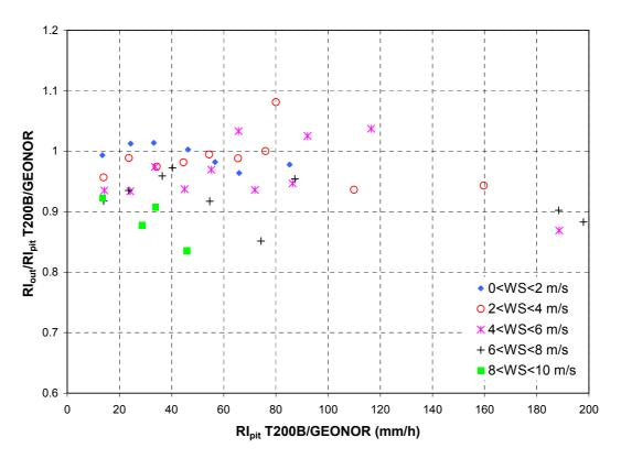
**Fig. 50:** 1-min T200B-GEONOR RI. RI<sub>out</sub>/RI<sub>pit</sub> vs RI<sub>pit</sub>; RI is divided in groups according to the wind speed conditions, then divided in groups of intensity and averaged inside each group.
