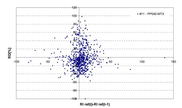
**5min RI scatter plot**: Comparison between 5-min averages of rainfall intensity measured by PP040-MTX and reference intensity. The uncertainty lines are calculated according to the procedure described in *Final Report, sec. 5*.3.2-*5*.3.3.
