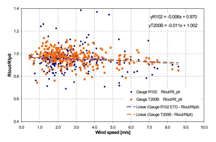
Fig. 47: Ratio between 5-min RI measured by the pit and RI measured by the identical gauge outside the pit.
