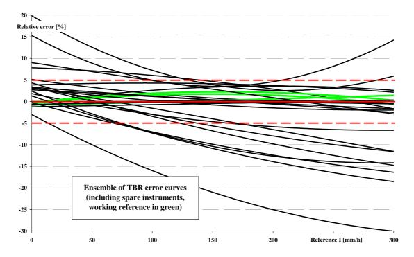
**Fig. 15**: Ensemble of the error curves obtained in the laboratory phase for all Tipping-bucket rain gauges, including the spare instruments, compared with the  $\pm 5\%$  uncertainty limits.
