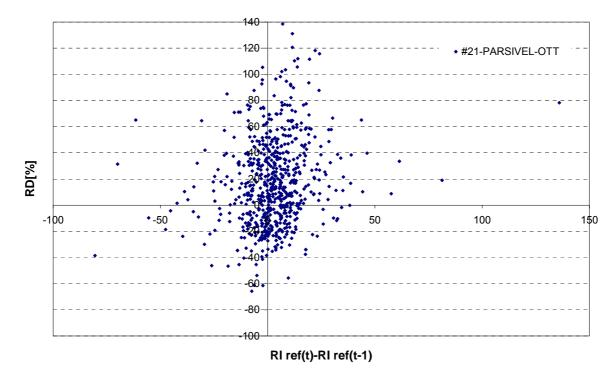
**5min RI scatter plot**: Comparison between 5-min averages of rainfall intensity measured by PARSIVEL OTT and reference intensity. The uncertainty lines are calculated according to the procedure described in *Final Report, sec.* 5.3.2-5.3.3.
