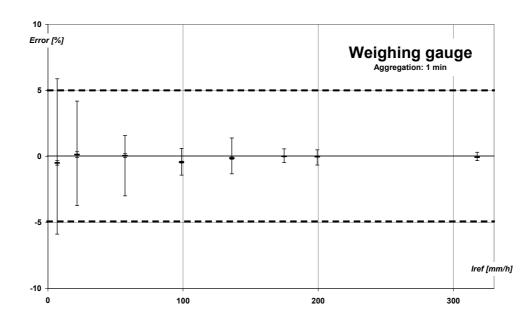
Fig. 14 (a), (b): Sample pit gauge TBR and WG instruments showing very good performance at the oneminute aggregation scale.
