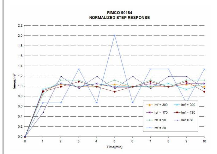
The "saw" response is mainly due to the measurement resolution.
