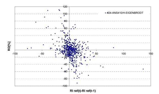
**5min RI scatter plot**: Comparison between 5-min averages of rainfall intensity measured by ANS410/H EIGENBRODT and reference intensity. The uncertainty lines are calculated according to the procedure described in *Final Report, sec.* 5.3.2-5.3.3.
