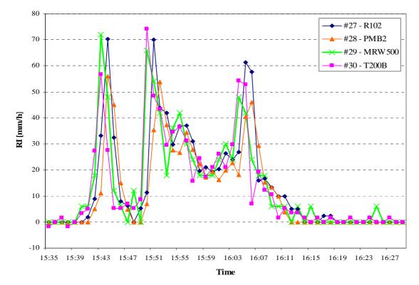
Fig. 38: Example of rainfall event: rainfall intensity measured by the working reference gauges.
