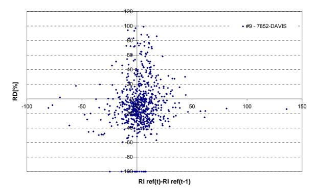
**5min RI scatter plot**: Comparison between 5-min averages of rainfall intensity measured by Rain Collector II- DAVIS and reference intensity. The uncertainty lines are calculated according to the procedure described in *Final Report, sec.* 5.3.2-5-3-3.
