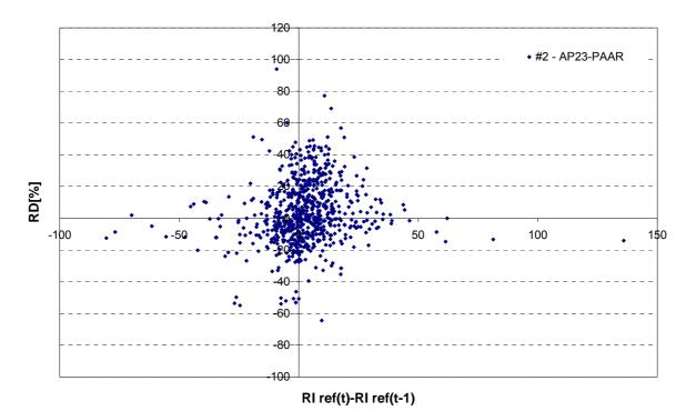
**5min RI scatter plot**: Comparison between 5-min averages of rainfall intensity measured by AP23-PAAR and reference intensity. The uncertainty lines are calculated according to the procedure described in *Final Report, sec. 5.3.2-5.3.3.*
