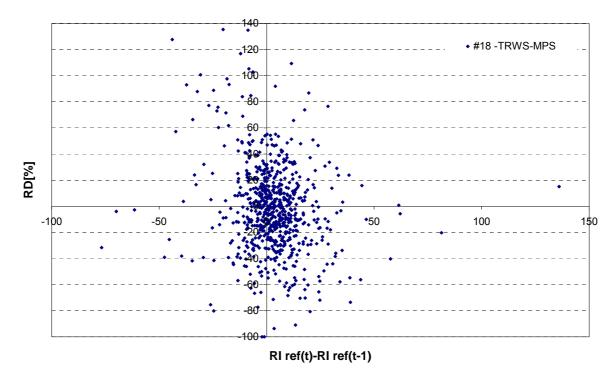
**5min RI scatter plot**: Comparison between 5-min averages of rainfall intensity measured by TRWS MPS and reference intensity. The uncertainty lines are calculated according to the procedure described in *Final Report, sec. 5.3.2-5.3.3.*
