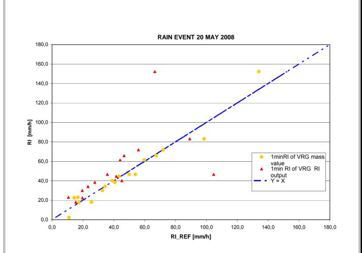
(1min RI of Vaisala VRG through mass value (orange circles) and through RI output (red triangles) are plotted versus the 1min REFERENCE RI. The Y=X line is reported to compare the results).
