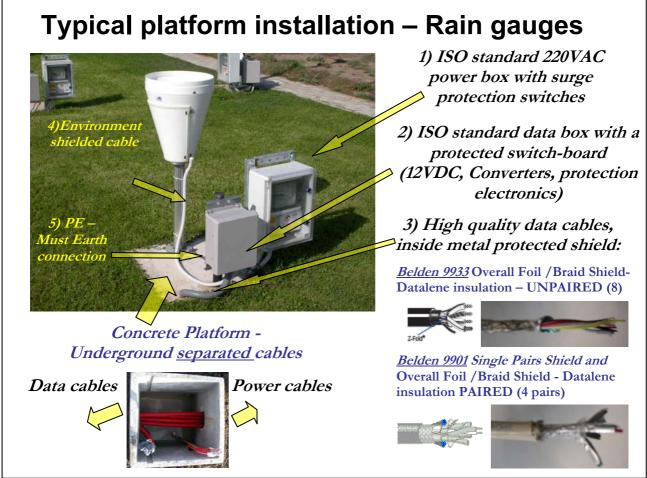
Fig. 11: The setup of the installation platforms and cabling.
