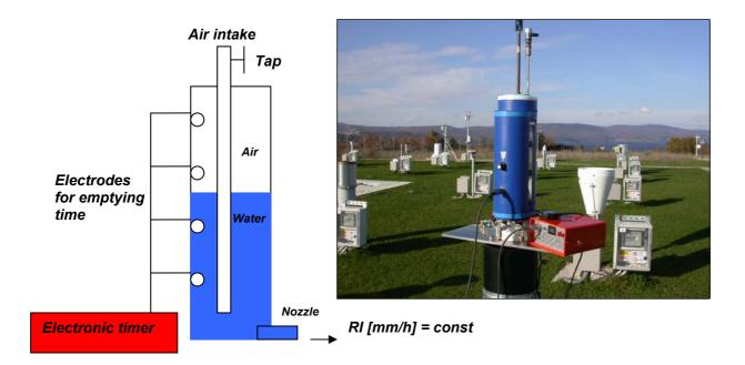
Fig. 24: The Portable Field Calibrator: the simplified scheme and the field setup during the Field Calibration at Vigna di Valle, Italy.
