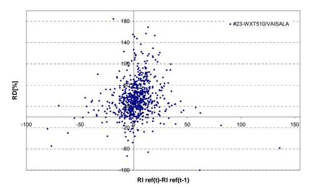
**5min RI scatter plot**: Comparison between 5-min averages of rainfall intensity measured by WXT510 VAISALA and reference intensity. The uncertainty lines are calculated according to the procedure described in *Final Report, sec.* 5.3.2-5.3.3.
