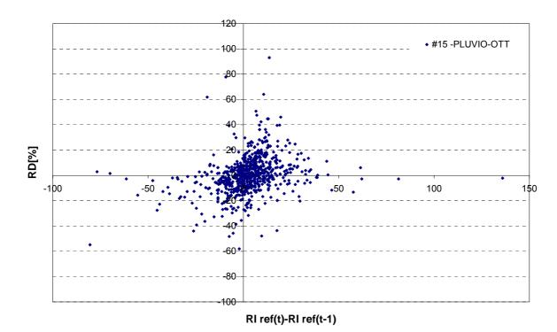
**5min RI scatter plot**: Comparison between 5-min averages of rainfall intensity measured by PUVIO-OTT and reference intensity. The uncertainty lines are calculated according to the procedure described in *Final Report, sec. 5*.3.2-*5*.3.3.
