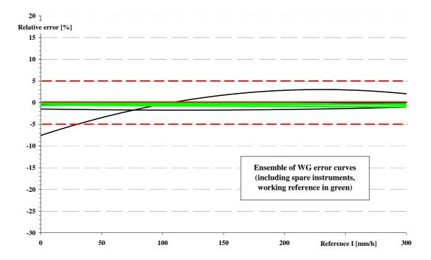
**Fig. 16**: Ensemble of the error curves obtained in the laboratory phase for all weighing gauges, including the spare instruments, compared with the ±5% uncertainty limits.
