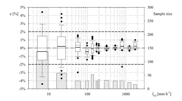
Fig. 21: One-minute variability for a sample WG observed performance and the size of the sample used for calculation of the statistics at each reference intensity.
