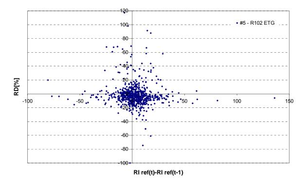
**5min RI scatter plot**: Comparison between 5-min averages of rainfall intensity measured by R 102-ETG and reference intensity. The uncertainty lines are calculated according to the procedure described in *Final Report, sec. 5.3.2-5-3-3.*
