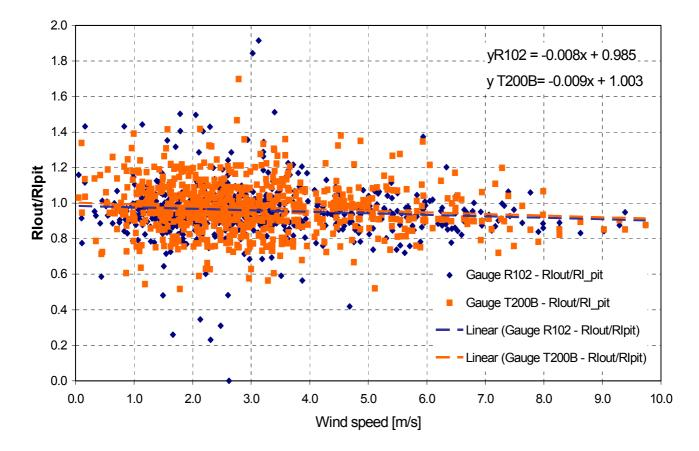
Fig. 46: Ratio between 1-min RI measured by the pit and RI measured by the identical gauge outside the pit.
