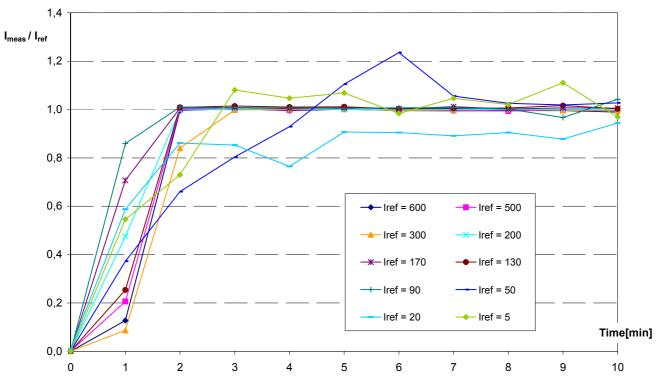
**Fig. 23**: Sample results from a step response test where the response curve for each single reference intensity is normalized and superimposed for better comparison.
