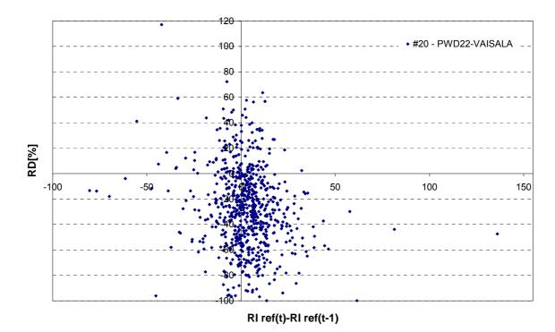
**5min RI scatter plot**: Comparison between 5-min averages of rainfall intensity measured by PWD22 VAISALA and reference intensity. The uncertainty lines are calculated according to the procedure described in *Final Report, sec.* 5.3.2-5.3.3.
