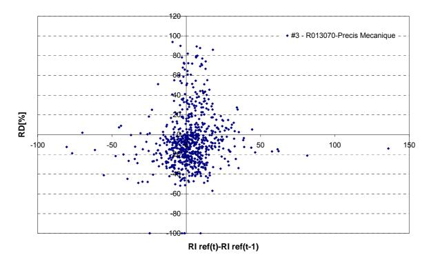
**5min RI scatter plot**: Comparison between 5-min averages of rainfall intensity measured by R01 3070 Precis Mecanique and reference intensity. The uncertainty lines are calculated according to the procedure described in *Final Report, sec.* 5.3.2-5.3.3.
