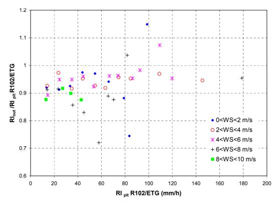
**Fig. 51:** 1-min R102-ETG RI. RI<sub>out</sub>/RI<sub>pit</sub> vs RI<sub>pit</sub>; RI divided in groups according to the wind speed conditions, then divided in groups of intensity and averaged inside each group.
