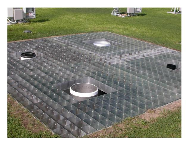
Fig. 3: The realization of the Reference Rain Gauge Pits at Vigna di Valle, Italy (2007).
