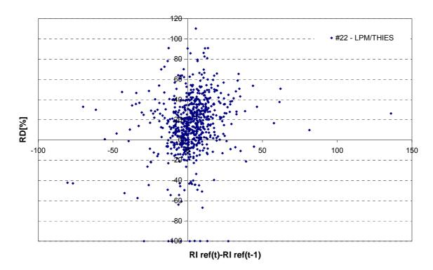
**5min RI scatter plot**: Comparison between 5-min averages of rainfall intensity measured by LPM-THIES and reference intensity. The uncertainty lines are calculated according to the procedure described in *Final Report, sec. 5*.3.2-*5*.3.3.
