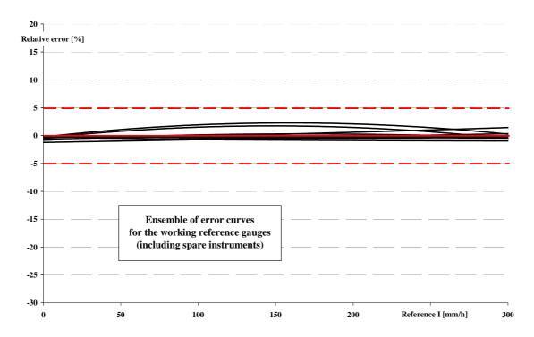
**Fig. 17**: Ensemble of the error curves obtained in the laboratory phase for the working reference gauges, including the spare instruments, compared with the  $\pm 5\%$  uncertainty limits.
