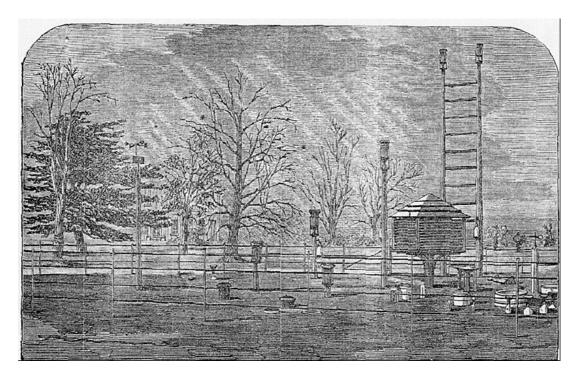
**Fig. 1**: Experiments to investigate the effect of measurement height on rainfall measures (by Symons in 1862) as quoted by Goodison et al., 1998.
