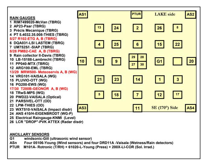
Fig. 10: Instrument positioning
