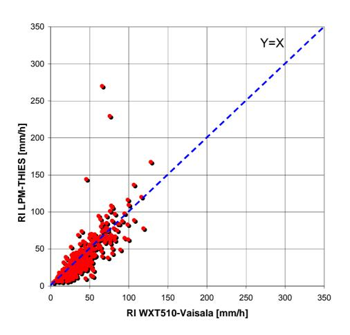
Apart from really few outliers, the experimental points in the plots show a very comparable behaviour. It means that the measuring principle adopted by the optical disdrometers gives the same results with respect to the reference RI, though the manufacturer's calibration procedures are totally different.
